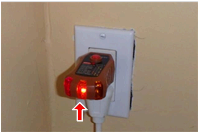
13.3 Item 14(Picture) The inspector noticed hot and neutral reversed receptacles scattered through out the house
